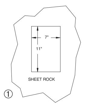
STEP 1: Cut 7" x 11" Hole in the Sheetrock.
